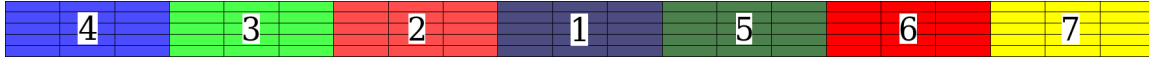
Figure 7.3: Simplified example of the balanced cantilever method - FE mesh with segment description.
