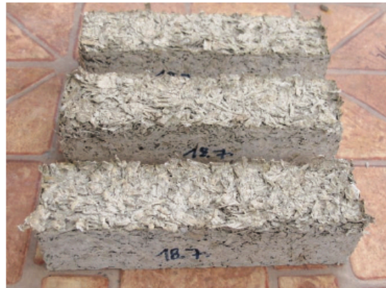
Figure 10. Samples of wood shavings concrete, which was used as a floor structure filler in CS2
