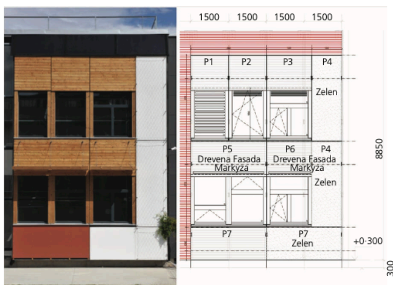
Figure 5. Photograph and schematic illustration of designed CWS from CS1 pilot installation on the south facade of the UCEEB, Czech Technical University, Prague. Source: Tywoniak et al. (2015)
