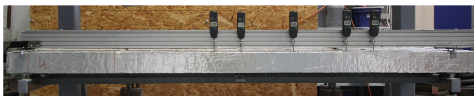
Fig. 5 Manual measurement of displacements at selected cross-sections using gauges
