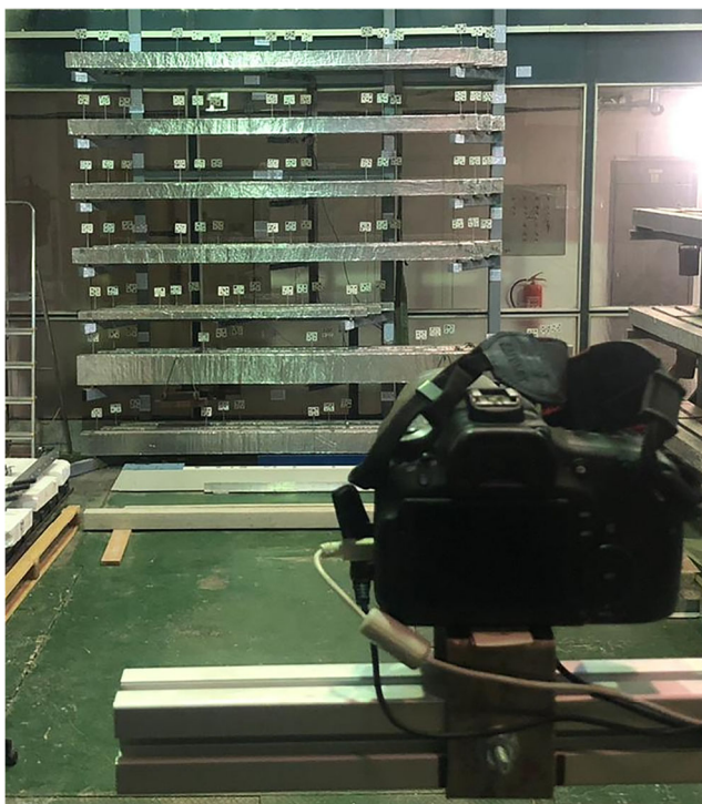
Fig. 4 Monitoring of displacements in the laboratory, the specimens and the DLSR camera connected to an external power source and a trigger
