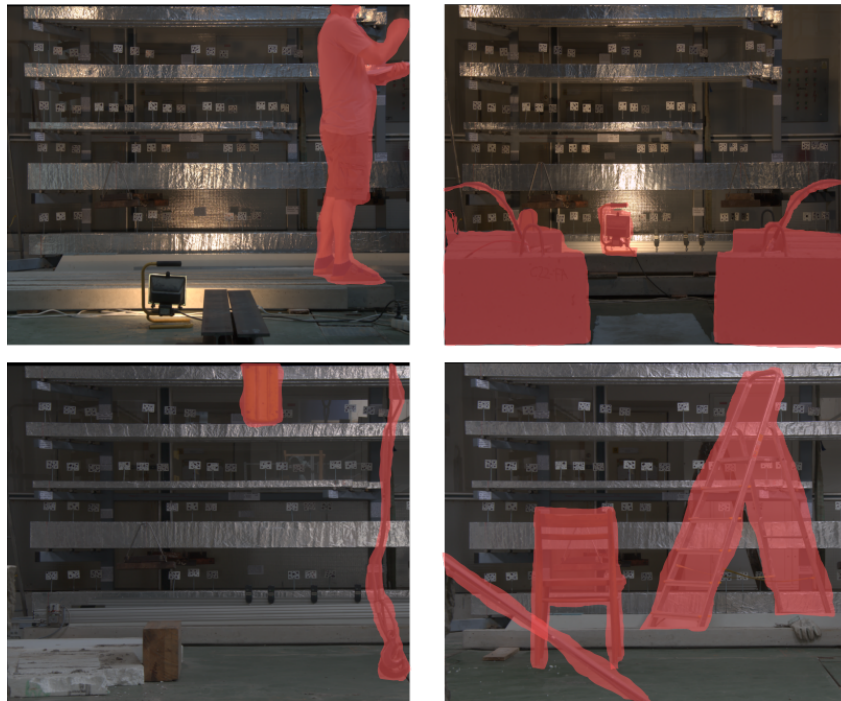
Figure 2.1: Obstructions in a camera view during a long-term experiment: a person (top-left), concrete blocks (top-right), a crane (bottom-left), and laboratory furniture (bottom-right).
