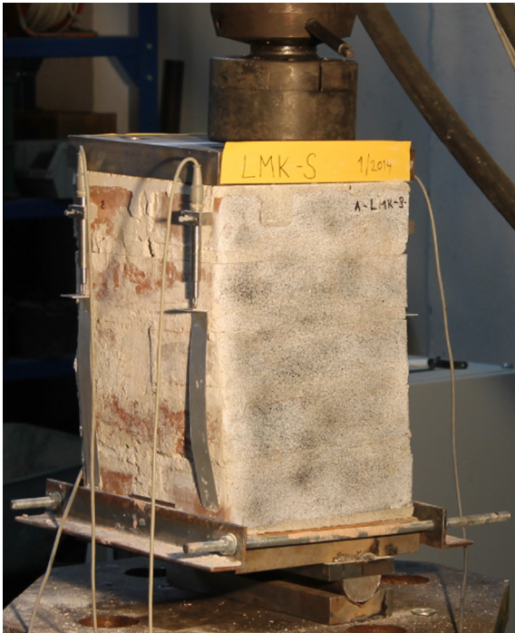
Fig. 5. Tested masonry pier subjected to the combination of compression and bending, introduced via eccentric loading and supporting.
