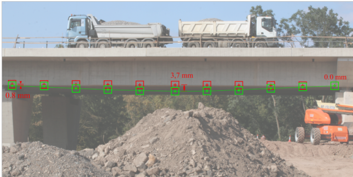
Figure 2.3: Bridge deflection measured from deck edge translation tracking using DFT-based correlation algorithms.
