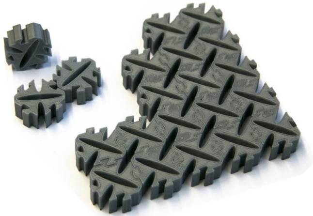
Fig. 1. Additively manufactured jigsaw puzzle tiles and partly disassembled auxetic aggregate with effective Poisson's ratio equal to -0.55 .
