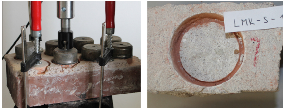
Fig. 2. Interface strength pull-out testing: experiment set-up (left) and the failure plane located within the mortar layer (right).
