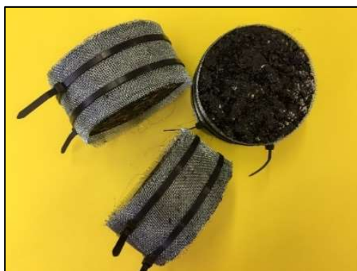
Figure 2. Test specimens wrapped by a steel mesh for PAV ageing procedure
