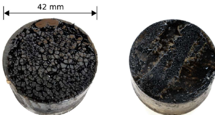
Fig. 7. Pull test specimens after cohesive (left) and adhesive (right) failure.
