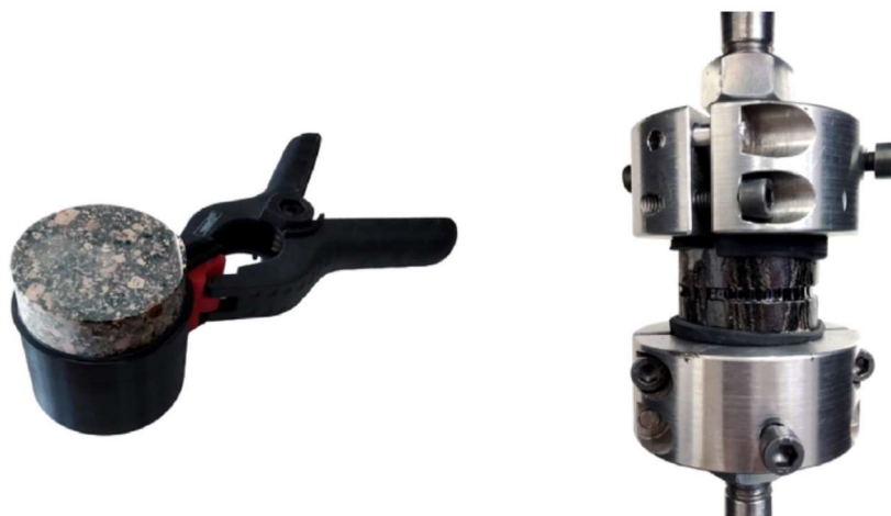
Fig. 3. Use of 3D-printed ring to avoid binder leakage during preparation of specimens for the direct-pull test (left) and clamping of a specimen failing in cohesion during the test (right).
