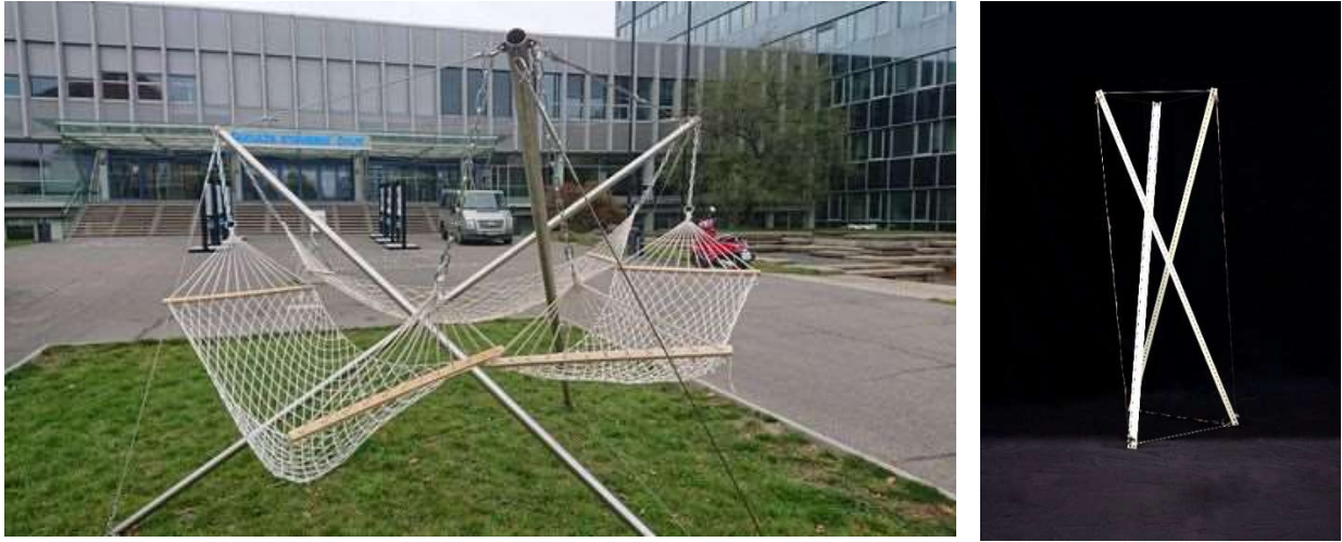
Fig. 1.1.3. Orthogonal Triangular Tensegrity Prism (models created by the author)
